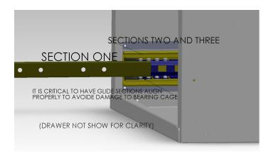
Both drawer slides need to line up properly for drawer insertion. When correctly aligned push drawer in all the way in and pull out to properly seat bearing cage.
