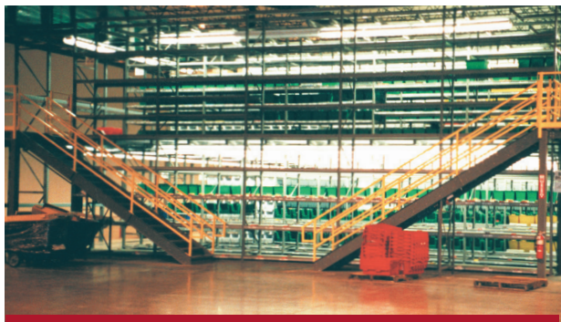
Multi-level Wide Span Pick Module
