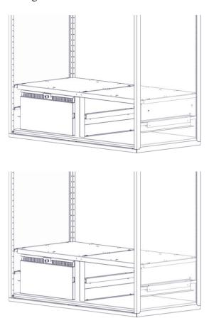
7K Install plastic glide rails to drawer guide rails using the provided screws. Then insert drawer onto the glide rails.
