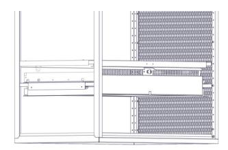
6E Install mounting rails for next drawer using the 8709 screws provided. 6F Install drawer guide rails using two rivets attached to mounting rails. 6G Install plastic glide rails to drawer guide rails using the provided screws. Then insert drawer onto the glide rails.
