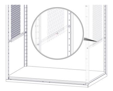
9B- Rivet seat to mounting rails in each corner as shown. For wooden seat install with lag bolts in each corner.
