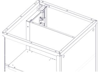
1C Install top clip to locker top rail and to doorframe using screw and rivets as shown.
