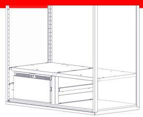
7I Install mounting rail for drawer using the 8709 screws provided
