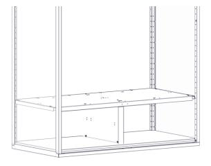
7D Install mounting rail for drawer using the 8709 screws provided.
