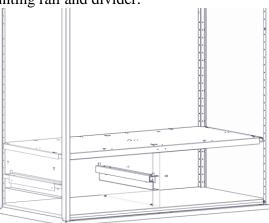
7F Install plastic glide rails to drawer guide rails using the provided screws. Next insert drawer onto the glide rails.
