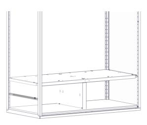
7E Install drawer guide rails using two rivets attached to mounting rail and divider.
