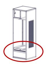
4A- Install the side mounting rails at the proper height locations using one screw in each corner. Rail height for footlocker is 13.9 inches from the outside bottom corner to the top of the rail. Two mounting rails required one on each side.
