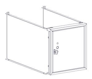
1B Install security box by sliding it onto the shelf in the appropriate position and secure it using four rivets as shown.
