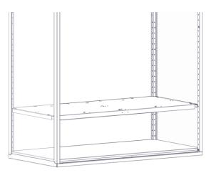
7C Install divider using rivets and screws. (Note it is critical to get this in the correct location for proper fit of side-by-side drawers.)
