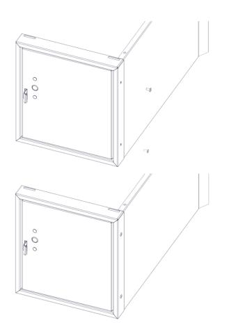
Optional side cover for hiding security box contents when locker sides are perforated.
