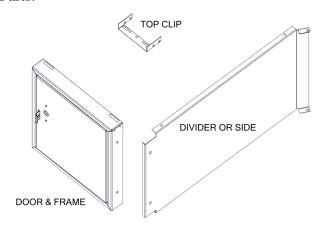
Step-1A Security box assembly and Installation Assemble the security box side to the frame using two rivets as shown. Note if locker sides are perforated and you need to hide security box contents then an additional side is required. Install this extra side on the opposite side facing the same way as the one in the image below.
