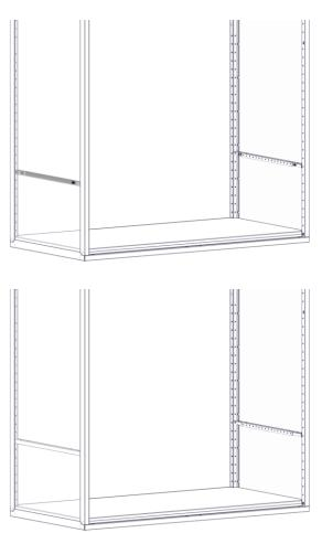
7B Install shelf on support rails using four rivets.
