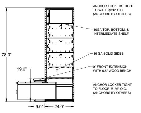
AVAILABLE AS WELDED OR KNOCK DOWN AVAILABLE SIZES: 18X24X78, 18X24X90, 24X24X78, 24X24X90 AVAILABLE DRAWER FRONT EXTENSIONS 9, 12 24 WIDE AVAILABLE WITH SINGLE OR DOUBLE DOOR AVAILABLE DOOR PERFORATIONS SOLID, LOUVER, DIAMOND AVAILABLE SIDE PERFORATIONS SOLID
