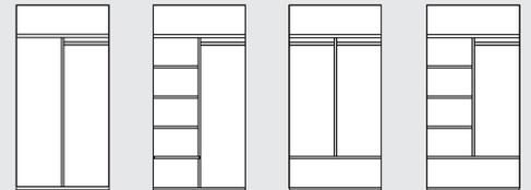
An optional center partition divides the locker space down the middle, allowing for half shelves or coat rods to be installed on either side.
