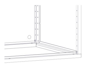
2E-Install 8709 screws to locker back at U cut locations (6-inch intervals) on each side.
