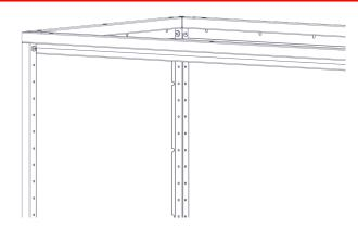
2D- Next install one screw into the locker top (which is on the ground) in each corner as shown.
