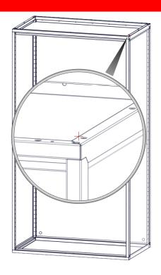
2C-2 Install one 8709 screw into each corner of the locker bottom as shown. Hint-This is where you will need the 6 inch #3 Philips bit extension
