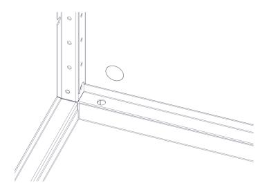
2B-2 With the back inserted install one 8709 screw on each side of the back about half way up. Note holes will align if the back is in the proper position.
