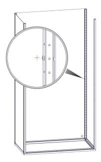
2C-1 In this step you are installing the locker bottom on top due to it being upside down. Be sure that the cast corner pieces align into the side frame channels
