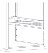
Step-8C- Insert two 8676 rivets through support rails and into front panel as shown.
