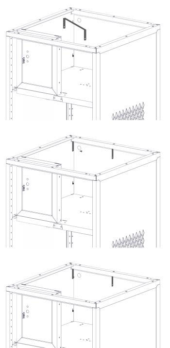
Step-3F Install second side with five 8676 rivets as shown. The locker side is on the inside of the frame. Note-If installing an L shelf do not rivet holes on the second security box side though the shelf, as the L shelf shares those holes.
