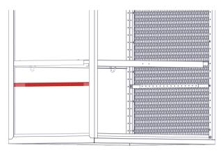
Step-14B Install plastic channels to drawer guide rails by sliding them onto drawer guide rails. Then attach using two 8721 screws in each rail.
