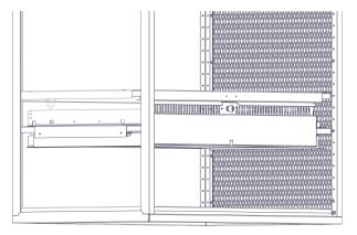
Step-14E Install mounting rails for next drawer using the 8709 screws provided.
