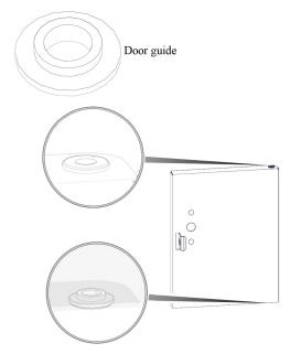
Step-3B Insert the 8676 rivets into the door guides in the top and bottom of door and into doorframe locking the door in place.
