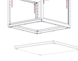
Step-10C Install seat using the four 8624 lag bolts into predrilled holes through support rails.
