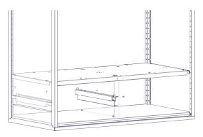
Step-15F Insert drawer onto the glide rails.
