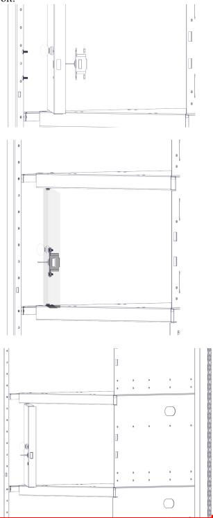
Step-7E Install doorstop angle by placing it in the correct position and inserting 8632 bolt and 7672 nuts to hold it in place as shown.
