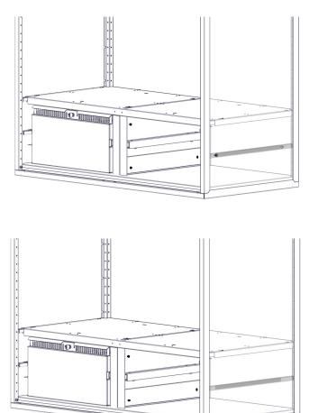
Step-15J Install drawer guide rails using two rivets attached to mounting rail and divider. Note plastic glides are attached prior to riveting drawer rails (see step 17E).
