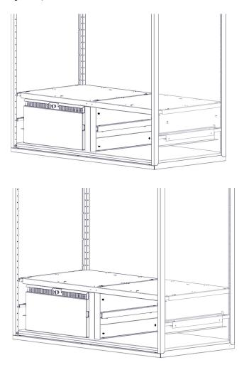
Step-15K Insert drawer onto the glide rails.
