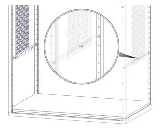
Step-10B Place wooden seat on top of rails in the correct position and mark it from the underside the mounting hole locations. One in each corner on the wooden bench through the support rails. Predrill those marked holes.
