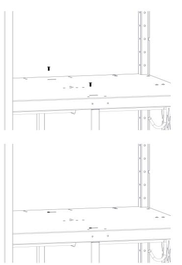
Step-5C Align bottom of partition in correct location on lower shelf or bottom. If a lower shelf is used, install with rivets or nut and bolt. If no lower shelf is used then install with self-tapping screws. (There are no guide holes on locker bottoms.)
