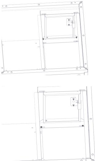
Step-3H- (Optional) Place 8676 rivet into the first side as shown.
