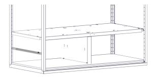
Step-15E Install plastic channels to drawer guide rails by sliding them onto drawer guide rails. Then attach using two 8721 screws in each rail.
