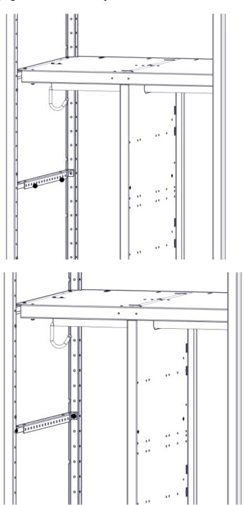
Step-6B Place side shelf on top of support rail, locate on shelf above, and insert four 8676 rivets to hold in proper location.
