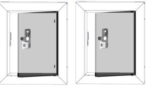
Step-3C Place security box side on top of the shelf at an angle as shown to allow attachment to door and frame. Attach to the frame using two 8676 rivets as shown. The side is on the inside of the frame. Note-This is done inside the locker on the shelf.
