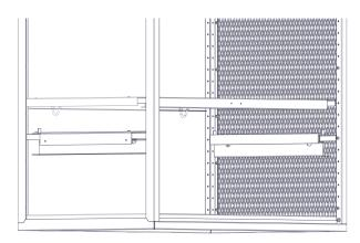
Step-14D Insert drawer onto the glide rails.
