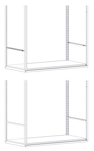
Step-15B Install shelf on support rails using four rivets.
