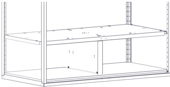
Step-15D Install mounting rail for drawer using the 8709 screws provided.
