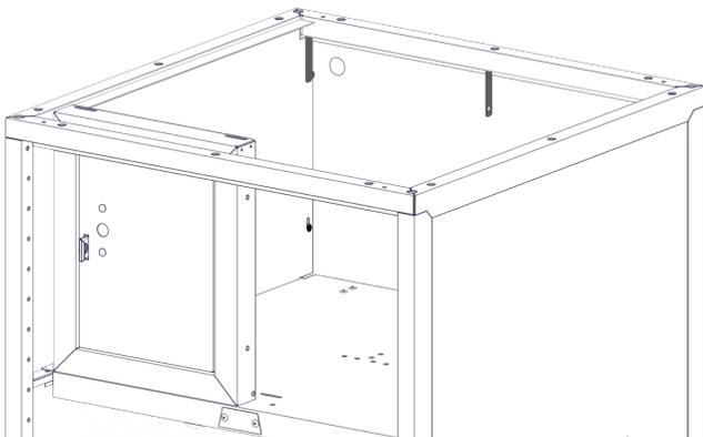
Step-3F Install second side with five 8676 rivets as shown. The locker side is on the inside of the frame.
