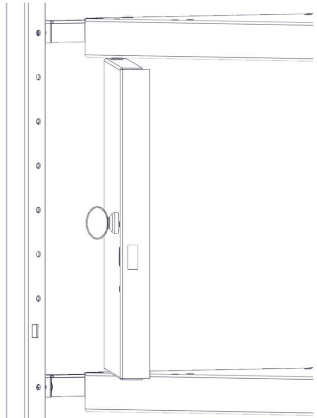
Step-7D Install lock by placing it from the backside of the door with the bolts 8632 entering from the front in the provided holes and install nuts 8672 on each bolt.
