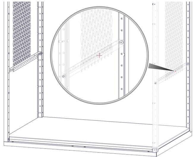
Step-9B- Rivet seat to mounting rails in each corner as shown.
