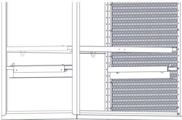
Step-14D Insert drawer onto the glide rails.
