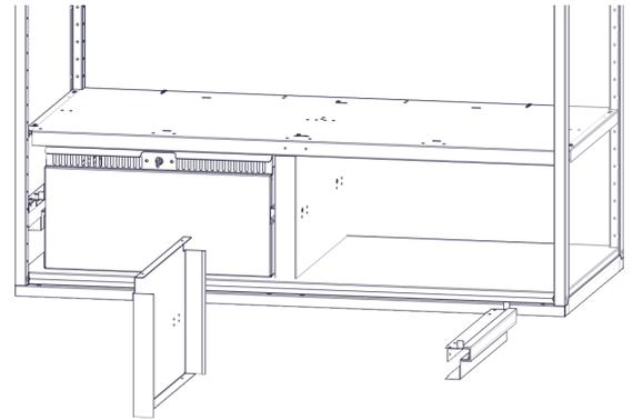
Step-15F Insert drawer onto the glide rails.
