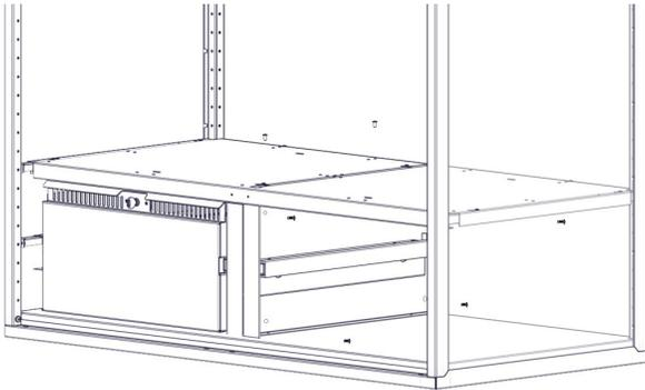
Step-15I Install mounting rail for drawer using the 8709 screws provided
