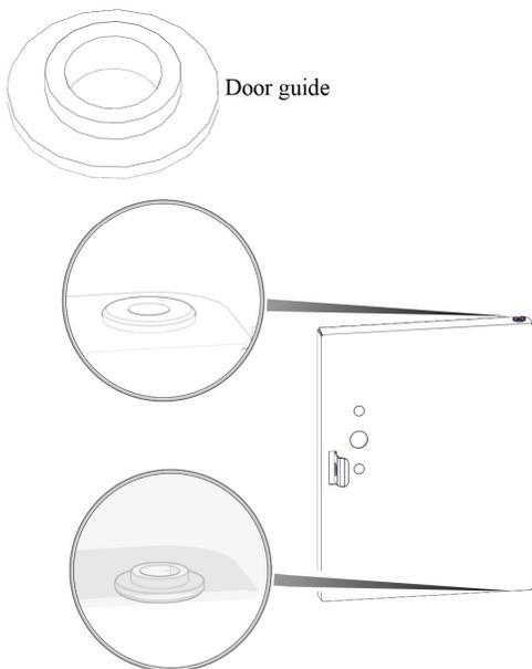
Step-3B Insert the 8676 rivets into the door guides in the top and bottom of door and into doorframe locking the door in place.
