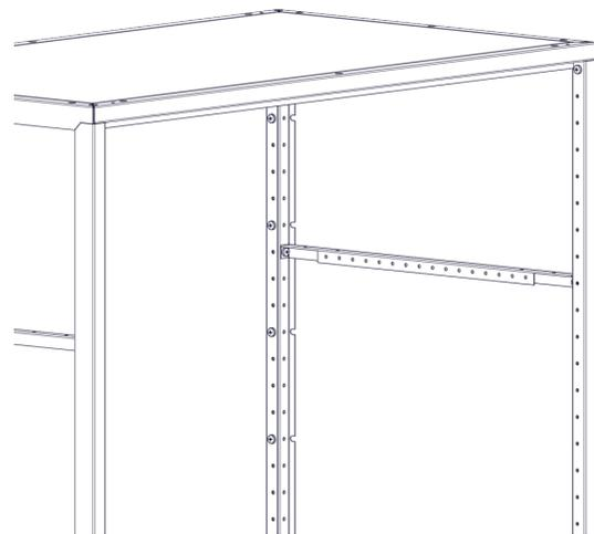
Step-2B Insert shelf and attach shelf to rails using one rivet in each corner. Be sure shelf position is completely to the back of the locker before riveting. Number plate holes should be facing locker opening.
