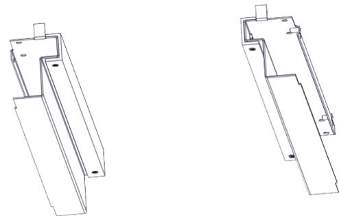
Step-15E Install drawer guide rails using two rivets attached to mounting rail and divider.
