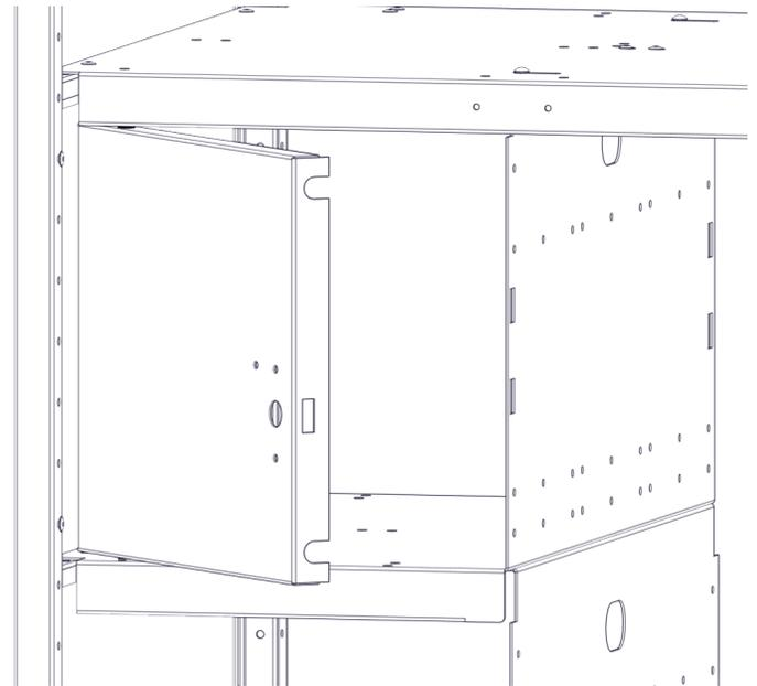
Step-7B Insert the 8676 rivets into the door guides in the top and bottom locking the door in place.
