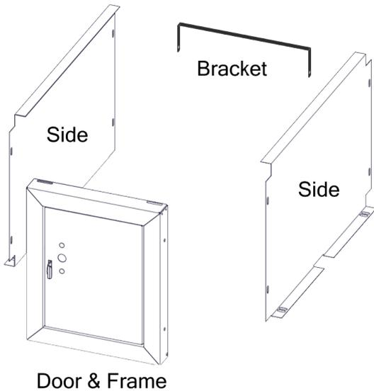
Step-3A Install door into frame with door guides as shown on the top and bottom of the door. Hold door guide in on the bottom until placed into the doorframe.
