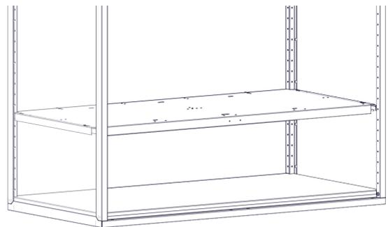
Step-15C Install divider using rivets and screws. (Note it is critical to get this in the correct location for proper fit of side-by-side drawers.)
