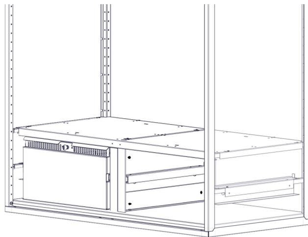
Step-15K Insert drawer onto the glide rails.
