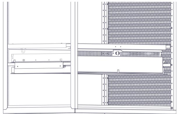
Step-14E Install mounting rails for next drawer using the 8709 screws provided.
