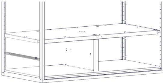
Step-15E Install plastic channels to drawer guide rails by sliding them onto drawer guide rails. Then attach using two 8721 screws in each rail.
