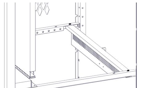
Step-8D- Next install the seat assembly using four rivets into the horizontal rails at the proper locations.
