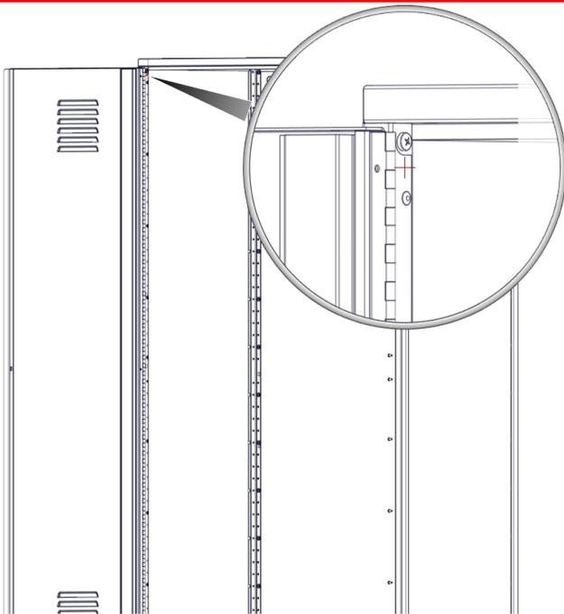
Step-19B Install number plate using 8671 rivets as shown.
