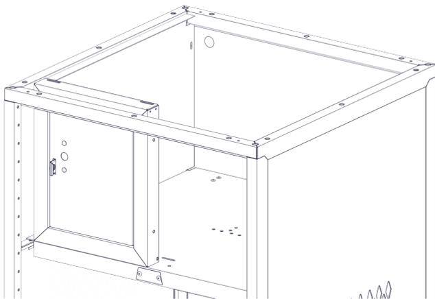
Step-3E Install rear bracket and install with 8676 rivet as shown.
