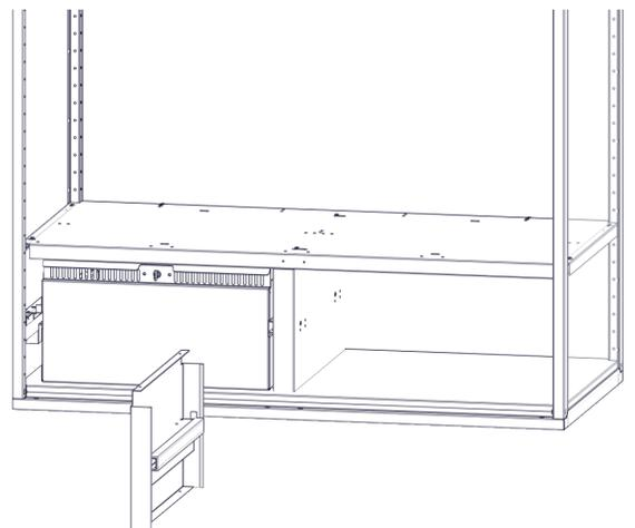
Step-15H Install divider using rivets. (Note it is critical to get this in the correct location for proper fit of side-by-side drawers.)
