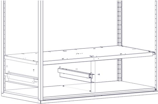
Step-15G Install guide rail to divider using rivets. Note plastic glides are attached prior to riveting drawer rails (see step 17E).
