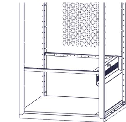
Step-8C- Insert two 8676 rivets through support rails and into front panel as shown.
