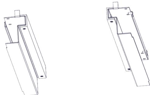
Step-14C Install drawer guide rails using two 8676 rivets each to mounting rails. The back hole should line up with the mounting rail back hole as shown.
