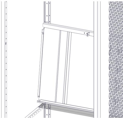
Step-8E- Now install the rubber bumpers on the seat and at proper height on the vertical posts.
