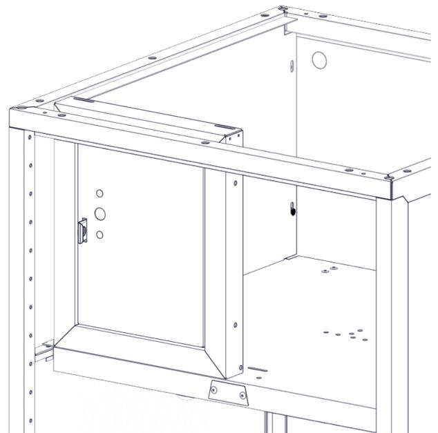
Step-3D Position door/frame and side to proper location and install 8676 rivet into bottom slot of side and into vertical frame.
