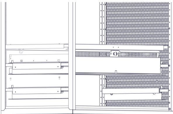
Step-14G Insert drawer onto the glide rails.
