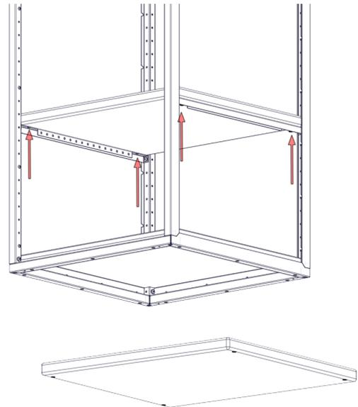
Step-10C Install seat using the four 8624 lag bolts into predrilled holes through support rails.
