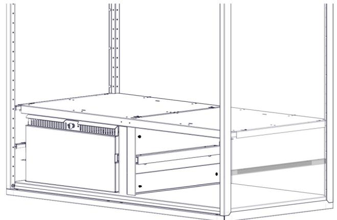
Step-15J Install drawer guide rails using two rivets attached to mounting rail and divider. Note plastic glides are attached prior to riveting drawer rails (see step 17E).
