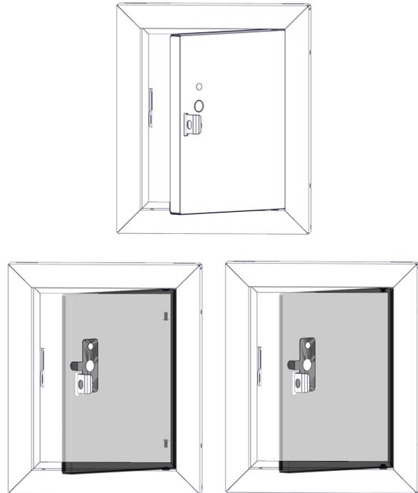
Step-3C Place security box side on top of the shelf at an angle as shown to allow attachment to door and frame. Attach to the frame using two 8676 rivets as shown. The side is on the inside of the frame. **Note- This is done inside the locker on the shelf.**
