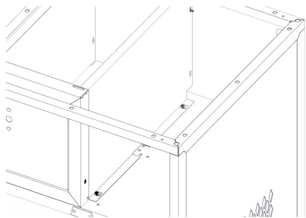
Step-3G Anchor door and frame to shelf using two 8676 rivets as shown.
