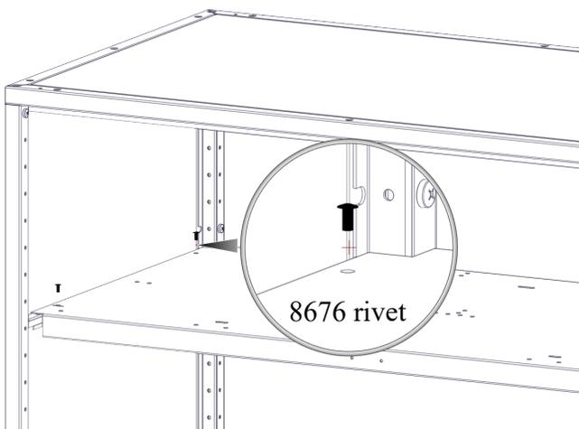
**STEP 3 – Assemble and install optional security box.**
