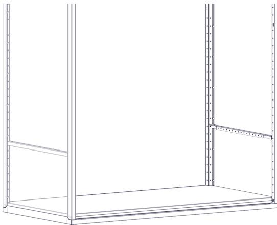
Step-15B Install shelf on support rails using four rivets.
