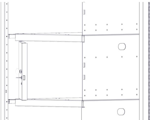
Step-7E Install doorstop angle by placing it in the correct position and inserting 8632 bolt and 7672 nuts to hold it in place as shown.
