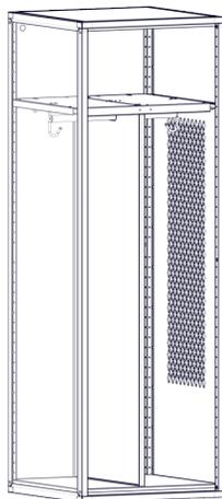
Step-5C Align bottom of partition in correct location on lower shelf or bottom. If a lower shelf is used, install with rivets or nut and bolt. If no lower shelf is used then install with self-tapping screws. (There are no guide holes on locker bottoms.)
