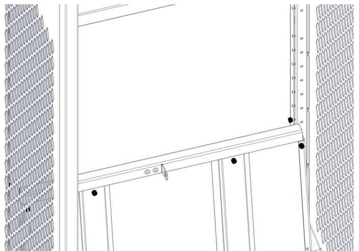
Step-8F- Now install the side channels using 8676 rivets on to the support rails as shown.
