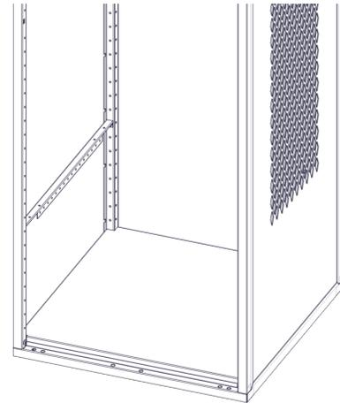
Step-8A- Install the side mounting rails at the proper height locations using one screw in each corner. Rail height for footlocker is 13.9 inches from the outside bottom corner to the top of the rail. Two mounting rails required one on each side.
