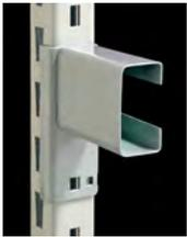
Rigidity beams provide lateral stability when steel shelves are used. A minimum of 2 pairs of beams is required per unit. They are constructed of 3" high steel channels with return flanges, with a beam end connector welded to each end.
