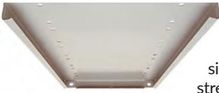
Clipper Conventional Flange Shelves are fabricated from 18 gauge cold rolled steel. All sides of the shelf are double flanged for added strength. The corners are lapped and welded for positive reinforcement. Shelves secure to posts with Penco's unique compression Clipper clip, or can be bolted. Shelves are punched for divider placement on alternating 1" and 2" centers. Reinforcing options are shown at right.
