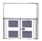
Step-22B Using 1.5 inch self-tapping screws go through the vertical frame channel at the rear of the locker and into the flange of the FEP. Use existing holes in the back and vertical channel for pilot holes. Screws spacing is 9-12 inches. Note Hold FEP firmly in place when installing self-tapping screws.
