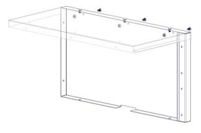
Step-3B Install left hand side to top using nut 7672, and bolt 8633 or rivets 8676.
