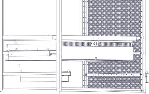
Step-14F Install drawer guide rails using two rivets attached to mounting rails. Note plastic glides are attached prior to riveting drawer rails (see step 16B).
