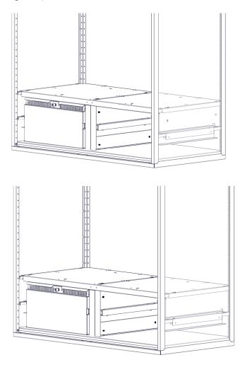
Step-15K Insert drawer onto the glide rails.
