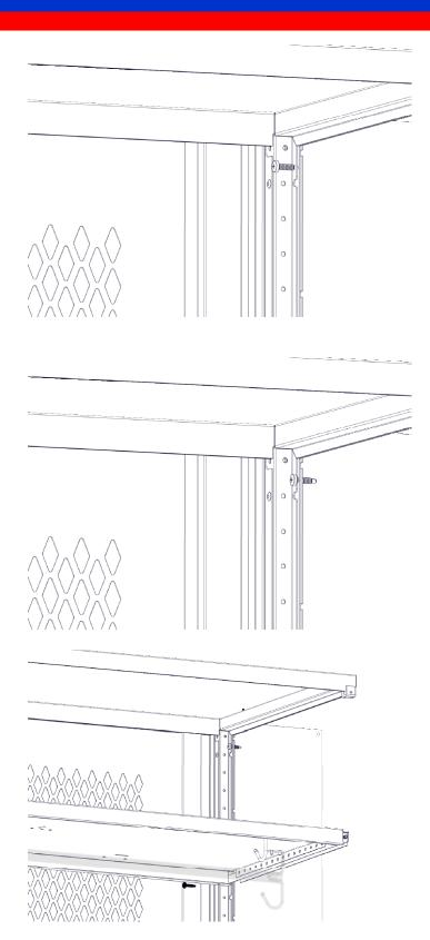
21C. Add additional self-tapping screws about every 9-12 inches to fasten filler to locker securely.
