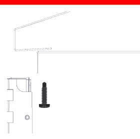
20C. Place self-tapping screw as close to the front channel as the screw head will allow. This will ensure penetration through the slope hood flange.
