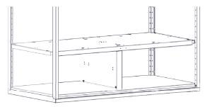
Step-15D Install mounting rail for drawer using the 8709 screws provided.
