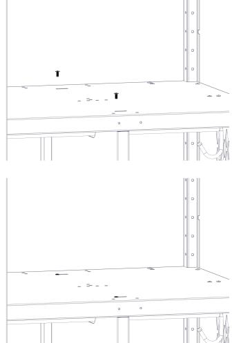
Step-5C Align bottom of partition in correct location on lower shelf or bottom. If a lower shelf is used, install with rivets or nut and bolt. If no lower shelf is used then install with self-tapping screws. (There are no guide holes on locker bottoms.)
