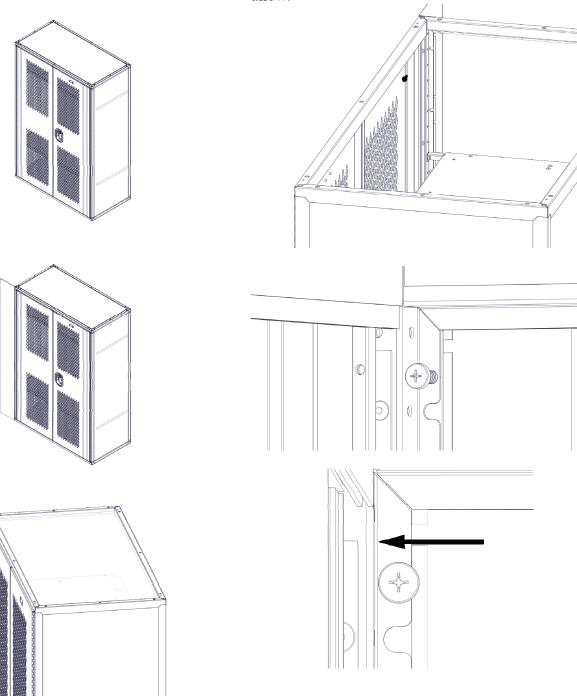
21B Use self-tapping screw to go through the flange of the vertical channel on the locker and into the flange of the vertical filler. The screw head should be, as close to the box channel as screw head will allow.
