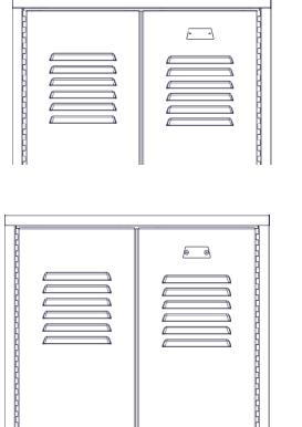
Door assembly is now complete. Anchor lockers to the floor and wall so they are plumb and level before use to ensure proper function.
