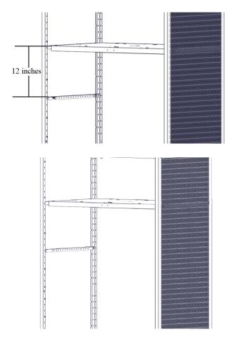
Step-4B Place L shelf on top of support rail and locate on shelf above and insert four 8676 rivets to hold in proper location.
