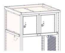
Step-3A Install right hand side to top using nut 7672, and bolt 8633 or rivets 8676.
