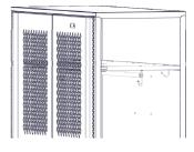
20B Align slope hood flush with the top frame channel on lockers and fasten with self-tapping screws (1" length)
