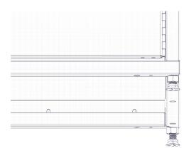
13E. Adjust rear right foot down until the doors are level across the top.
