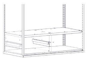
Step-15F Insert drawer onto the glide rails.
