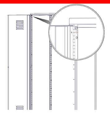
Step-19B Install number plate using 8671 rivets as shown.
