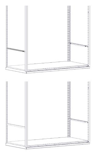
Step-15B Install shelf on support rails using four rivets.
