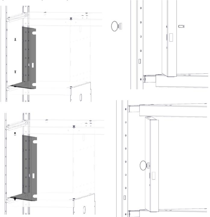
Step-7D Install lock by placing it from the backside of the door with the bolts 8632 entering from the front in the provided holes and install nuts 8672 on each bolt.
