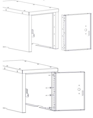
Step-3E Install door pull 60803Z to door using 8632 bolts and 8672 nuts.
