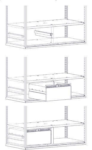
Step-15G Install guide rail to divider using rivets. Note plastic glides are attached prior to riveting drawer rails (see step 17E).
