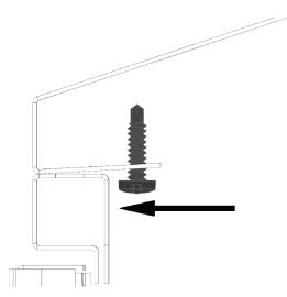
20D. Add self-tapping screws approximately every 12 inches to fasten slope hood securely.
