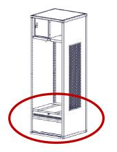
Step-8A- Install the side mounting rails at the proper height locations using one screw in each corner. Rail height for footlocker is 13.9 inches from the outside bottom corner to the top of the rail. Two mounting rails required one on each side.
