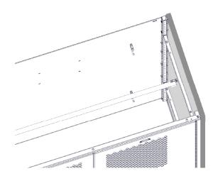
Step-22C Use 1 inch self-tapping screws to anchor FEP in the front. Install screws through flange on the vertical channel as shown below. Note install screw as close to vertical channel as screw head will allow.
